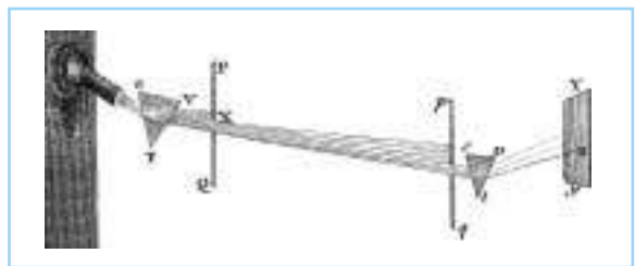
Figure 1.1 An eighteenth-century representation of Newton's Experimentum crucis . As the left-hand prism is rotated around its long axis, the beam selected by the two diaphragms is constant in its angle of incidence at the second prism. Yet the beam is refracted to different degrees at the second prism according to the degree to which it is refracted at the first. (From Nollet's Leçons de Physique Expérimentale ).
